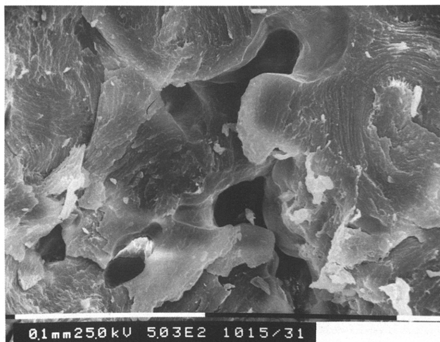
Fig. 7. Detail showing entrapment of air voids at the core/pseudogel boundary region of an HPMC tablet after 1 h hydration ( \times 500 ).
